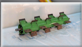
Feed accelerator with rubber paddles
