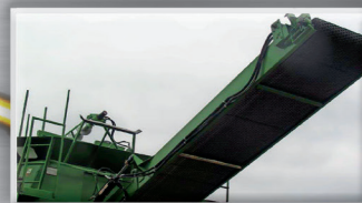
Unload conveyor 20' long with 30'' wide belt
