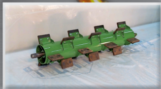
Feed accelerator with rubber paddles
