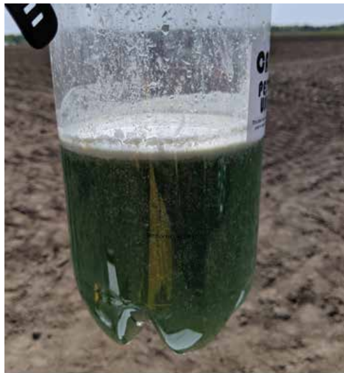
Figure 1. Flocculation resulting from the mixture of 10-34-0 fertilizer with fungicides evaluated in the in-furrow field trials.
